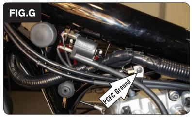
Secure the PCFC ground wire with the small ring lug to the common ground used for the throttle cable holder on the left side of the frame just rear of the ignition coil (Fig. G).
