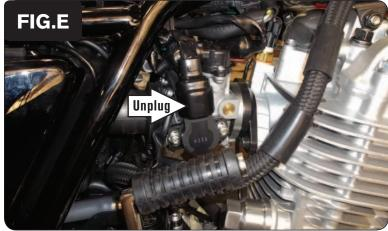
Unplug the stock BLACK 3-pin connector from the bike's Throttle Position Sensor on the right hand side of the throttle body (Fig. E).
