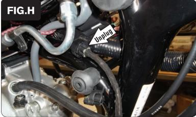
11 Trace the cable from the bike's stock O2 sensor in the exhaust to a BLACK 4-pin connector located on the right side of the frame and unplug this connector (Fig. H).
