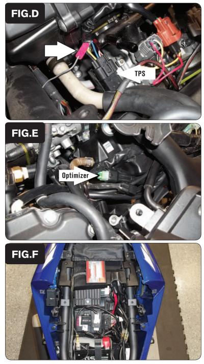
Using the supplied Posi-tap attach the GREY wire of the PCFC to the stock YELLOW wire of the bike's Throttle Position Sensor (Fig. D).
