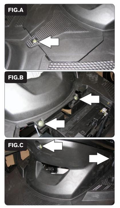
1 Remove the battery cover (Fig. A).
