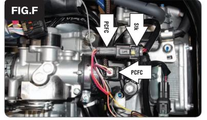
7 Plug the PCFC in-line of the stock injector and wiring harness (Fig. F).
