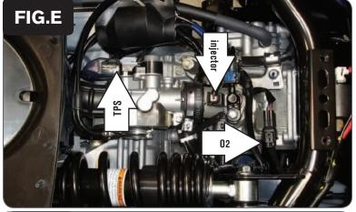
6 Unplug the Throttle Position Sensor, Injector and O2 from the main wiring harness (Fig. E).
