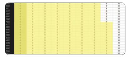
The PCFC for this model controls the stock closed loop area. This area is represented by the highlighted cells. The PCFC is designed to achieve a target AFR of 13.6:1. To use this PCFC you must retain your stock O2 sensor.
