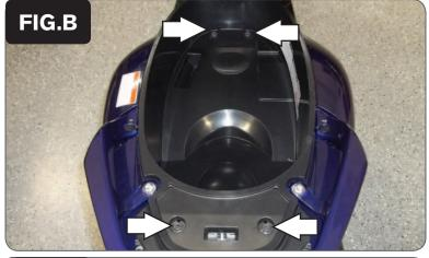
2 Remove the 4 bolts shown in Figure B and remove the storage trunk.
