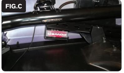
Install the PCFC to the left, inside of the bodywork (Fig.C). Use the supplied velcro to secure the module in place.
