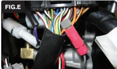
8 Using the supplied Posi-tap, attach the GREY wire of the PCV to the stock ORANGE wire of the main wiring harness plugged in at the ECU (Fig. E).
