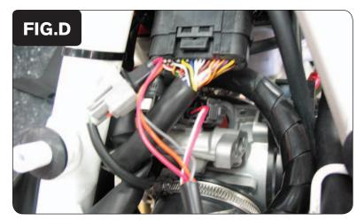
Plug the PCV harness in-line of the fuel injector and the stock wiring harness (Fig. D).
