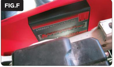
11 Using the supplied Velcro, attach the PCV module to the inside of the left side plastic body panel (Fig. F).
