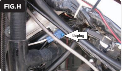
11 Locate and unplug the stock connectors for the bike's Ignition Coil (Fig. H).
