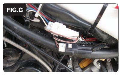
10 Plug the pair of WHITE 2-pin PCV connectors with BROWN colored wires in-line of the bike's stock Crank Position Sensor connectors (Fig. G).
