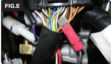
8 Using the supplied posi-tap attach the GREY wire from the PCV to the stock ORANGE/BLACK wire of the stock ECU connector (Fig. E).
