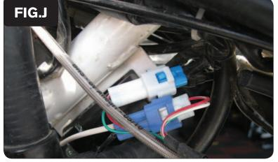
12 Plug the pair of WHITE 2-pin PCV connectors with RED and GREEN colored wires in-line of the bike's stock Ignition Coil connectors (Fig. J).
