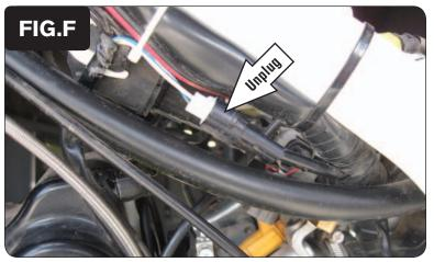
9 Locate and unplug the stock connectors for the vehicle's Crank Position Sensor (Fig. F).
