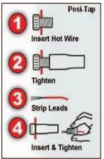
Attach the BROWN/WHITE wire of the PCV to the stock BLUE/YELLOW crank position wire.
