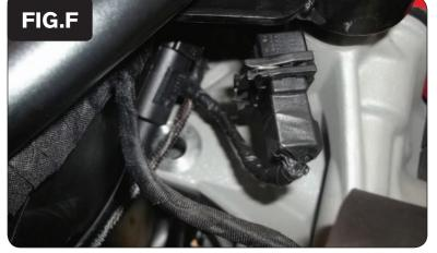
Plug the PCV wiring harness in-line of the TPS and the stock wiring harness (Fig. F).
