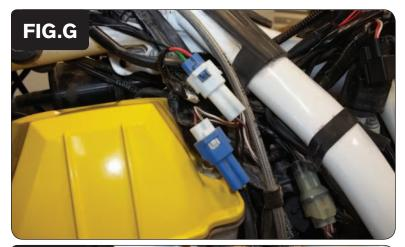
11 Plug the pair of WHITE 2-pin PCV connectors with BROWN colored wires in-line of the stock CPS connectors (Fig. G).
