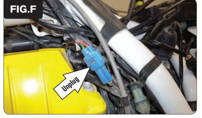
Unplug the bike's Crank Position Sensor connectors (Fig. F).
