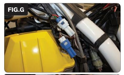
Plug the pair of WHITE 2-pin PCV connectors with BROWN colored wires in-line of the stock CPS connectors (Fig. G).
