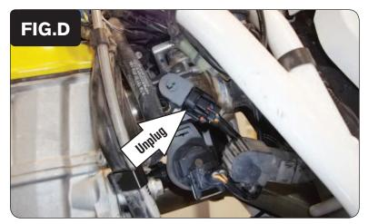
8 Unplug the Throttle Position Sensor located on the left side of the throttle body (Fig. D).
