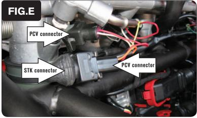
Plug the PCV harness in-line of the stock injectors and stock wiring harness (Fig. E).
