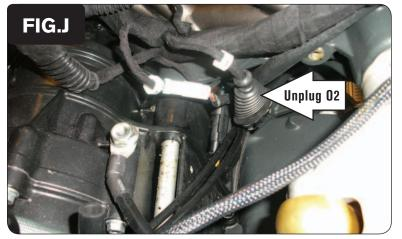
12 Unplug the stock O2 sensor from the wiring harness (Fig. J).
