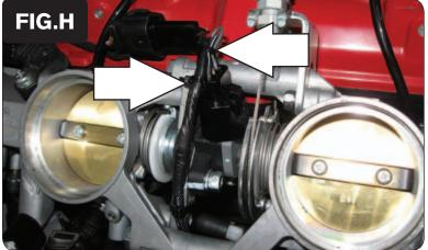
Plug the PCV wiring harness in-line with the bike's TPS and stock wiring harness. Use the 2 small zip ties to secure the wiring harness to the throttle bodies at the pointed locations (Fig. H). Check the throttle movement to ensure there isn't any interference.
