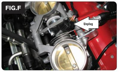
9 Locate and unplug the bike's Throttle Position Sensor between the 2nd and 3rd throttle bodies (Fig. F).
