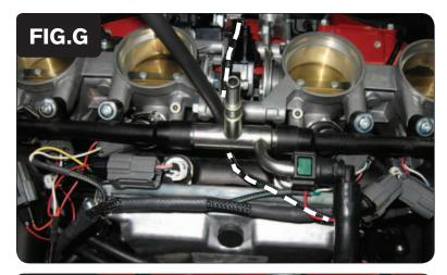
Route the pair of 3-pin TPS connectors of the PCV harness under the fuel rail and throttle body connecting bolt and up to the bike's TPS (Fig. G).
