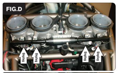
7 Unplug the stock wiring harness from each fuel injector (Fig. D).
