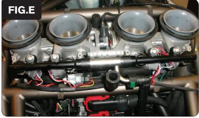
8 Plug the PCV in-line of the stock fuel injectors and wiring harness (Fig. E).
