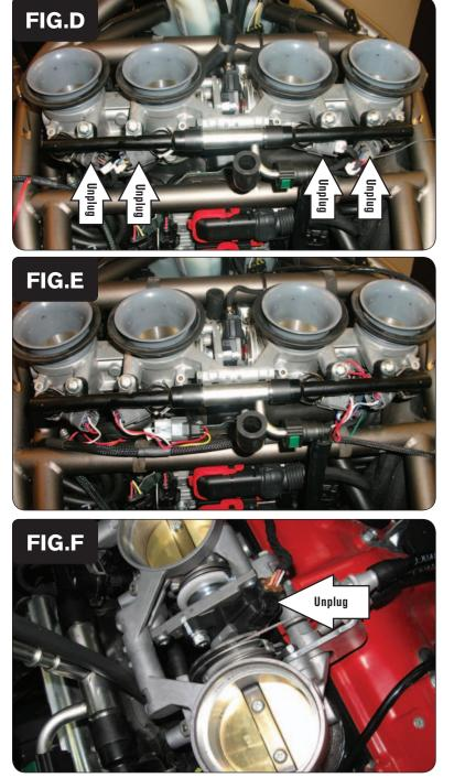
7 Unplug the stock wiring harness from each fuel injector (Fig. D).
