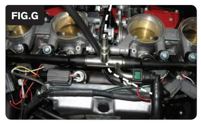
10 Route the set of 3 pin TPS connectors of the PCV harness under the fuel rail and throttle body connecting bolt and up to the bike's TPS (Fig. G).
