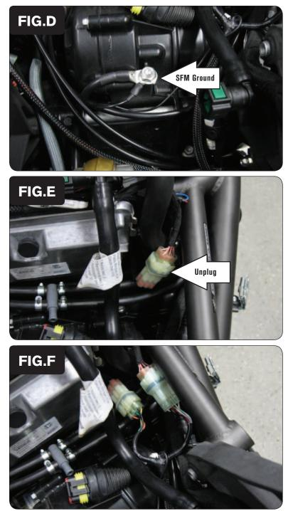
7 Attach the ground wire from the SFM wiring harness with the small ring eyelet to the stock ground bolt on top of the engine case (Fig. D).
