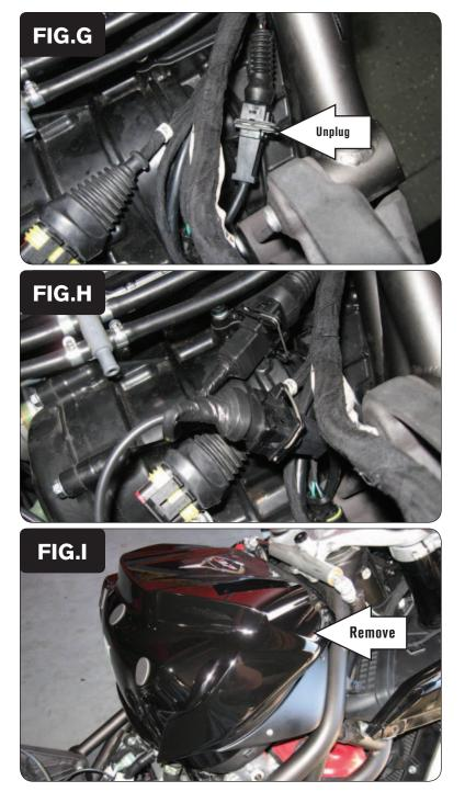
10 Locate the bike's crank position sensor connectors inside the right hand side of the frame (Fig. G).
