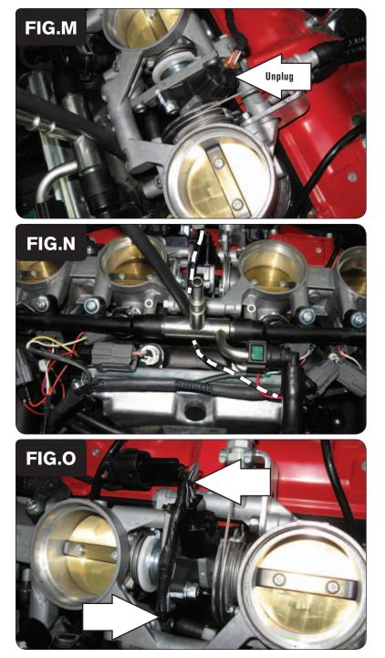
16 Locate and unplug the bike's throttle position sensor located between the 2nd and 3rd throttle bodies (Fig. M).
