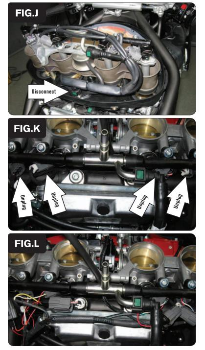
13 Once the airbox cover is removed, take the air filter out of it and disconnect the intake ducts from the front sides of the airbox. Disconnect the fuel line and electrical connectors at the bottom rear of the airbox (Fig. J). The entire airbox assembly should be able to lift off of the throttle bodies at this point.
