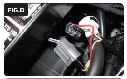
Plug the pair of PCV connectors with YELLOW colored wires PCV in-line of the stock wiring harness and the rear fuel injector (Fig. D).
