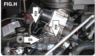
12 Plug the pair of 3-pin connectors on the PCV wiring harness in-line of the stock wiring harness and TPS (Fig. H).
