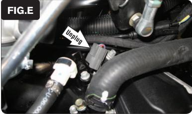
7 Unplug the stock wiring harness from the front fuel injector (Fig. E).
