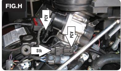
12 Plug the PCV connectors in-line of the stock wiring harness and TPS (Fig. H).
