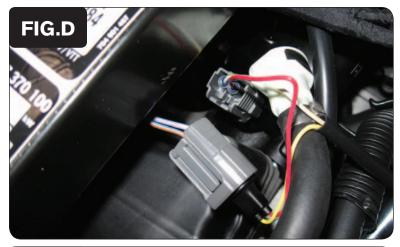
Plug the YELLOW colored wires from the PCV in-line of the stock wiring harness and the rear fuel injector (Fig. D).
