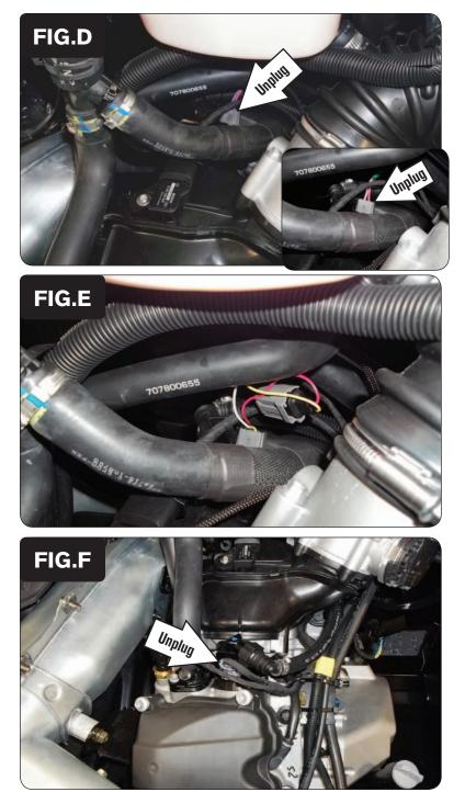
Unplug the stock wiring harness from the front cylinder fuel injector (Fig. D).
