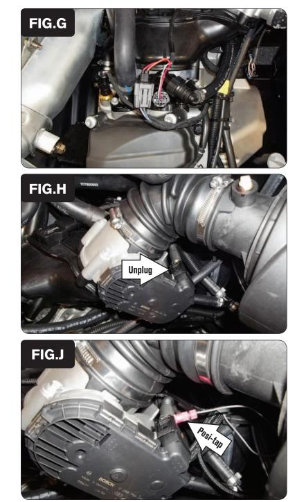
8 Plug the pair of PCV connectors with YELLOW colored wires in-line of the rear cylinder fuel injector and the stock wiring harness (Fig. G).
