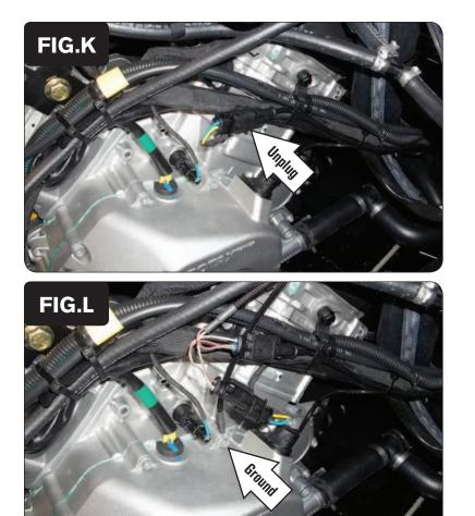
12 Unplug the stock Crank Position Sensor connectors (Fig. K).
