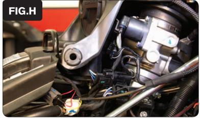
11 Plug the PCV connectors in-line of the stock wiring harness and TPS (Fig. H).
