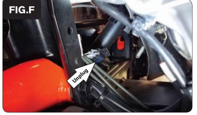
7 Locate and unplug the stock O2 sensor connector (Fig. F).
