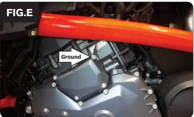
6 Secure the PCV ground wire with the small ring lug to the engine cover bolt shown in Figure E.
