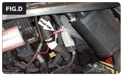
Use the supplied Posi-tap to attach the PCV RED wire to the stock ORANGE/GREEN wire of the GREY 6-pin connector near the ECU (Fig. D).
