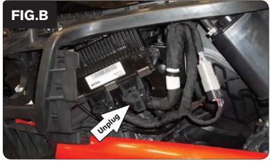
2 Unplug the rear most ECU connector (Fig. B).
