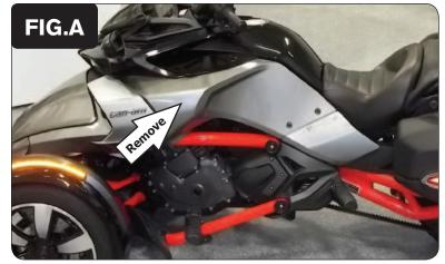
Remove the left side panel to expose the ECU compartment above the engine (Fig. A).
