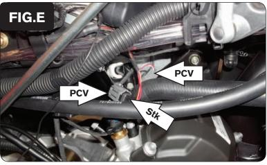
6 Plug the PCV in-line of the stock injector and wiring harness (Fig. E).
