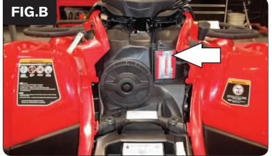
Using the supplied velcro secure the PCV to the back of the airbox (Fig. B). 3
