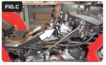
Route the PCV harness down towards the throttle body (Fig. C).
