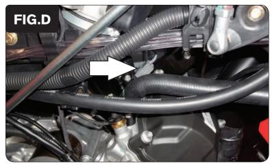
5 Unplug the stock fuel injector connector (Fig. D).
