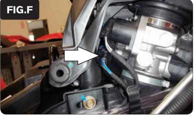
7 Unplug the stock Throttle Position Sensor connector (Fig. F).
