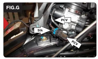
Plug the connectors from the PCV in-line of the TPS and stock wiring harness (Fig. G).
