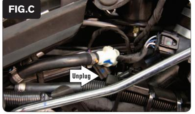
5 Unplug the stock wiring harness from the rear fuel injector (Fig. C).
