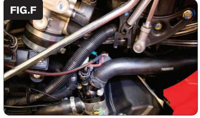
Plug the pair of leads on the PCV harness with ORANGE colored wires in-line of the front fuel injector and stock wiring harness (Fig. F).
