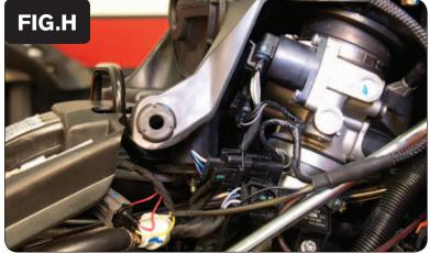
11 Plug the PCV connectors in-line of the stock wiring harness and TPS (Fig. H).
