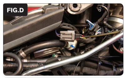
Plug the pair of leads on the PCV harness with YELLOW colored wires in-line of the rear fuel injector and stock wiring harness (Fig. D).
