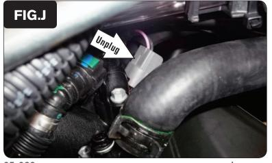
10 Unplug the front cylinder fuel injector (Fig. J).
