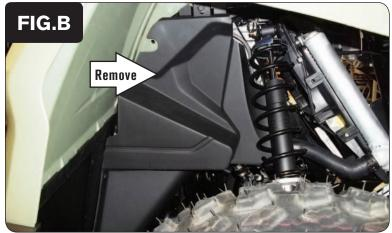
2 Remove the splash guard inside the front right fender well (Fig. B).
