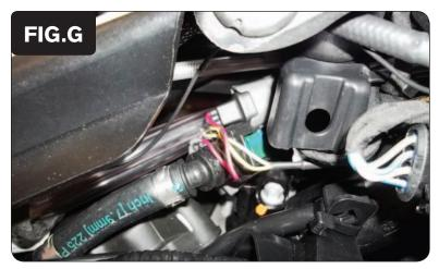
Plug the pair of PCV 2-pin connectors with YELLOW colored wires in-line of the rear cylinder fuel injector and the stock connector (Fig. G).
