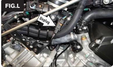
12 Locate and unplug the stock Crank Position Sensor connectors (Fig. L).
