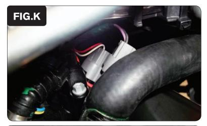
11 Plug the pair of 2-pin PCV connectors with ORANGE colored wires in-line of the front cylinder fuel injector and the stock connector (Fig. K).
