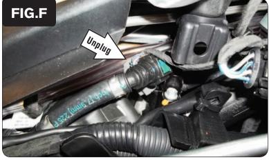
7 Unplug the rear cylinder fuel injector (Fig. F).
