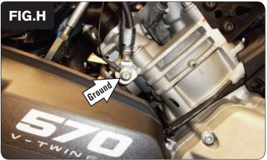
9 Route and secure the PCV ground wire with the small ring terminal to the stock common ground bolt on the rear cylinder head (Fig. H).
