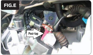
8 Using the supplied Posi-tap, attach the GREY wire of the PCV to the stock RED wire of the TPS wiring harness (Fig. E).
