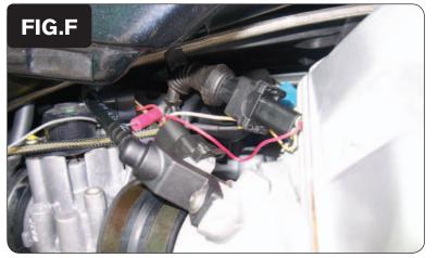
Plug the pair of PCV leads with YELLOW colored wires in-line of the RIGHT fuel injector and the stock wiring harness (Fig. F).
