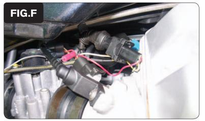
Plug the pair of PCV leads with YELLOW colored wires in-line of the RIGHT cylinder fuel injector and the stock wiring harness (Fig. F).
