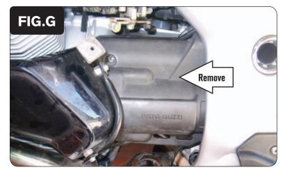
12 Remove the plastic cover on the left hand side of the engine (Fig. G).
