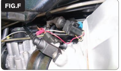
11 Plug the pair of PCV leads with YELLOW colored wires in-line of the RIGHT cylinder fuel injector and the stock wiring harness (Fig. F).
