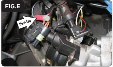
9 Using the supplied Posi-tap, attach the GREY wire of the PCV to the stock RED wire of the TPS wiring harness (Fig. E).
