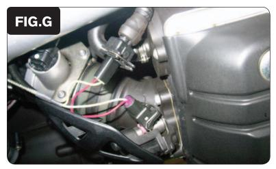
9 Plug the pair of PCV leads with YELLOW colored wires in-line of the RIGHT fuel injector and the stock wiring harness (Fig. G).
