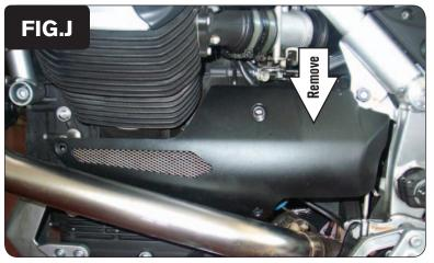
13 Remove the BLACK plastic engine cover on the left side (Fig. J).
