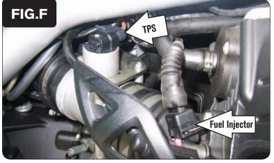
Unplug the stock wiring harness from the RIGHT fuel injector (Fig. F).
