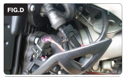
Plug the pair of PCV leads with ORANGE colored wires in-line of the LEFT fuel injector and the stock wiring harness (Fig. D).
