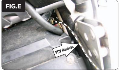
Route the pair of PCV leads with YELLOW colored wires to the RIGHT throttle body. Go inside of the frame tube as shown in Figure E.
