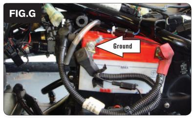
13 Secure the ground wire of the PCV wiring harness with the 6mm ring lug to the negative (-) terminal of the bike's battery (Fig. G).
