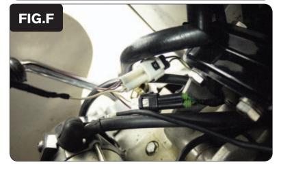
Plug the pair of PCV wiring harness leads with BROWN colored wires in-line of the stock Crank Position Sensor connectors (Fig. F).
