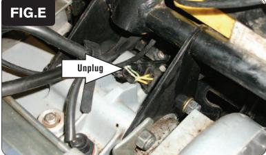
11 Locate and unplug the bike's Crank Position Sensor connectors (Fig. E).
