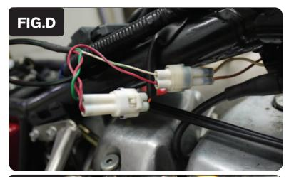
10 Plug the pair of PCV wiring harness leads with the GREEN colored wires in-line of the bike's Ignition Coil and stock wiring harness (Fig. D).
