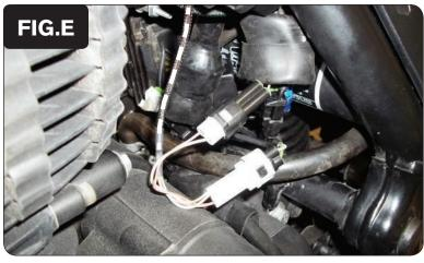
Plug the pair of PCV connectors with BROWN colored wires in-line of the stock Crank Position Sensor connectors (Fig. E).
