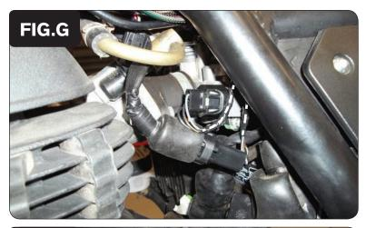
Plug the pair of 3-pin PCV connectors with GREY wires in-line of the Throttle Position Sensor and the stock wiring harness (Fig. G).
