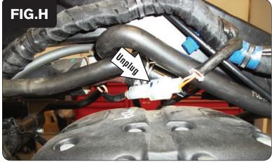
11 Unplug the stock Ignition Coil connectors (Fig. H).
