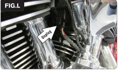
Locate and unplug the stock wiring harness from the bike's Ignition Coil (Fig. L).
