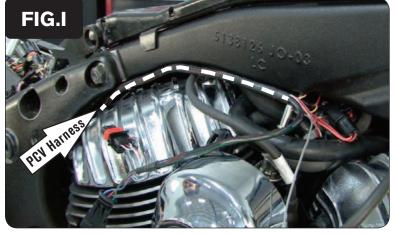
12 Route the other PCV wiring harness branch forward towards the engine. Go through the opening in the frame directly in front of the battery, then over the top of the rear cylinder, between the rear cylinder valve cover and the frame, towards the fuel injectors located between the two cylinders under the frame.
