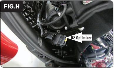
Plug the other supplied O2 Optimizer into the bike's stock wiring harness in-place of the stock front O2 sensor (Fig. H).
