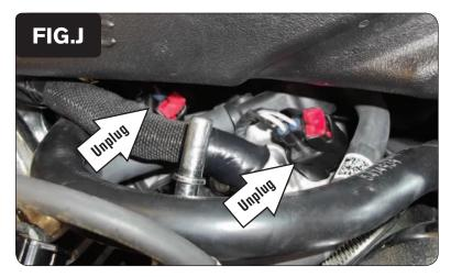
13 Locate and unplug the stock wiring harness from the front and rear Fuel Injectors (Fig. J).
