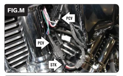
17 Route the pair of 3-pin connectors from the PCV down to the Ignition Coil and plug these connectors in-line of the Ignition Coil and the stock wiring harness (Fig. M).
