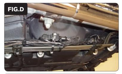
7 Plug the PCV wiring harness in-line of the stock CPS connectors (Fig. D).
