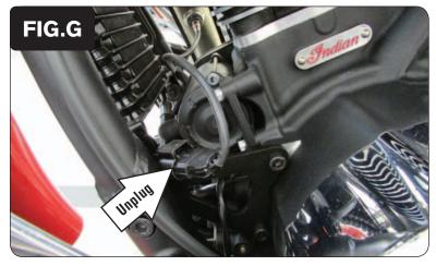
Locate and unplug the stock connector for the bike's front cylinder O2 sensor (Fig. G).
