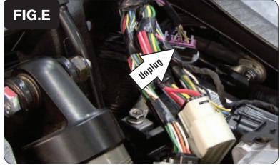
Under the seat, locate and unplug the stock connector for the bike's rear cylinder O2 sensor (Fig. E).
