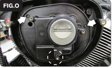
20 Remove the air filter backing plate (Fig. O).
