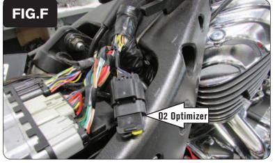
Plug one of the supplied O2 Optimizers into the bike's stock wiring harness in-place of the stock O2 sensor (Fig. F).
