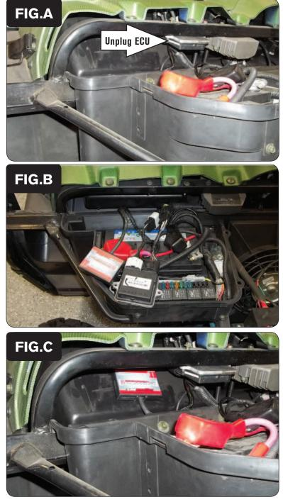
1 Locate and unplug both of the vehicle's stock ECU connectors (Fig. A).
