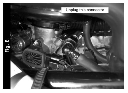
8 Unplug the stock wiring harness from the injector (Fig. E).
