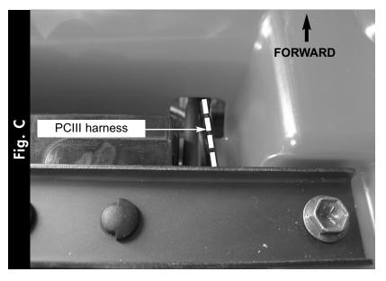
5 Route the PCIII harness under the battery bracket and through the hole in the fender (Fig. C).
