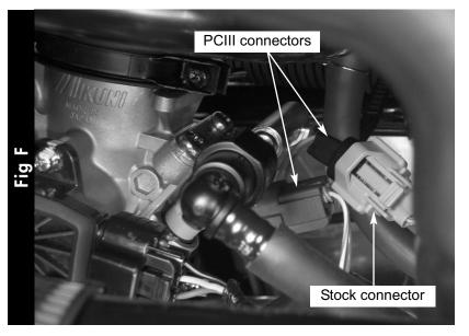
Plug the connectors from the PCIII in-line of the stock wiring harness and fuel injector (Fig.F).
