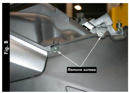
4 Remove the body cover by removing the 2 screws on each side of the panel (Fig. B)
