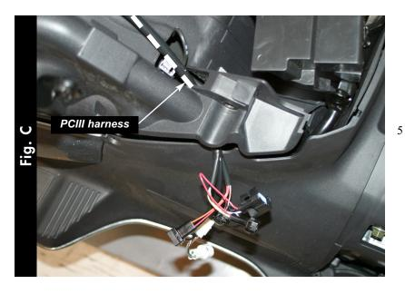
The battery tray panel will need to be lifted up so the PCIII harness can be routed through it (Fig. C).
