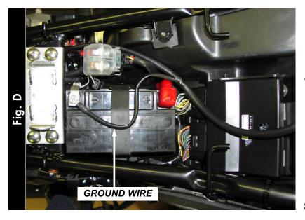
7 Attach the ground wire from the PCIII to the NEGATIVE side of the battery (Fig. D).
