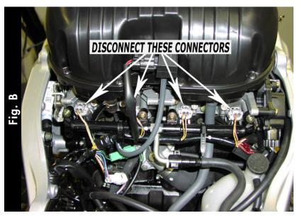
5 Unplug the stock wiring harness from each injector (Fig. B).
