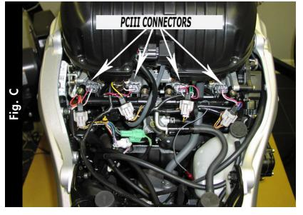
Plug the connectors from the PCIII inline of the stock injectors and the stock wiring harness (Fig.C).
