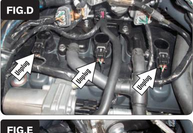
7 Unplug the stock wiring harness from each coil stick (Fig. D).
