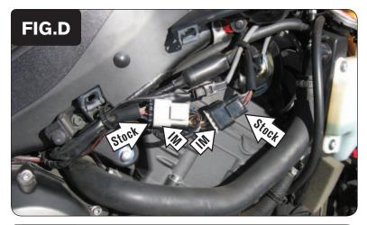
6 Plug the Ignition Module connectors in-line of the stock wiring harness (Fig. D).
