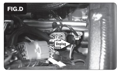
9 Locate and unplug the stock Crank Position Sensor connectors (Fig. D).
