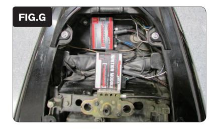
12 Plug the CAN link cable into one of the expansion ports of the Ignition Module and the other end into one of the expansion ports of the PCV module.
