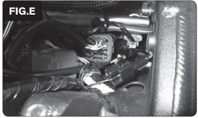
Plug the pair of 2-pin connectors of the Ignition Module in-line of the stock Crank Position Sensor connectors (Fig. E).
