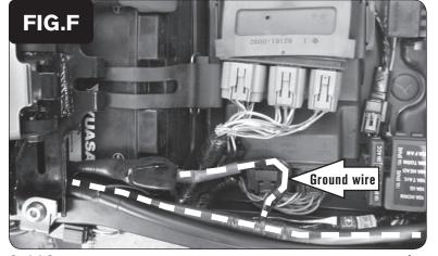
11 Secure the ground wire from the Ignition Module with the ring terminal to the negative (-) post of the bike's battery (Fig. F).
