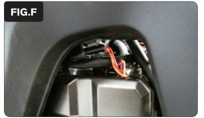
You might find it easiest to rotate the cylinder #1 coil stick to the left and make your connections through the frame on the left side, as shown in Figure F.
