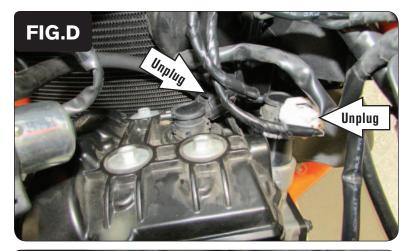
At the front cylinder head, unplug the stock BLACK connector from the Primary Front Cylinder Ignition Coil at the center of the head. Also unplug the stock WHITE connector from the Secondary Front Cylinder Ignition Coil at the side of the head (Fig. D).
