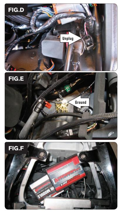
9 Locate and unplug the stock Crank Position Sensor connectors (Fig. D).
