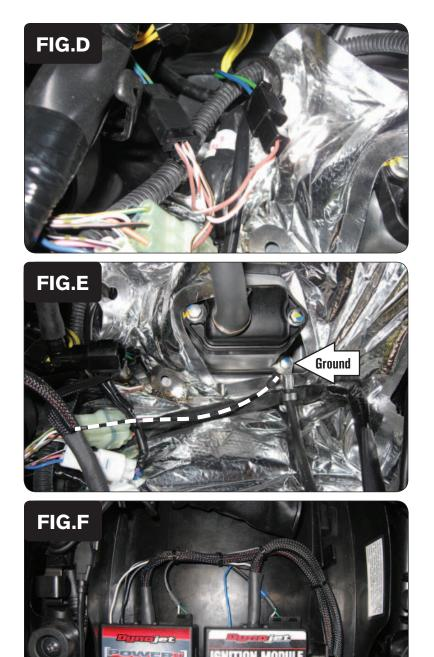
Plug the pair of connectors from the Ignition Module with BROWN colored wires in-line of the stock Crank Position Sensor connectors (Fig. D).
