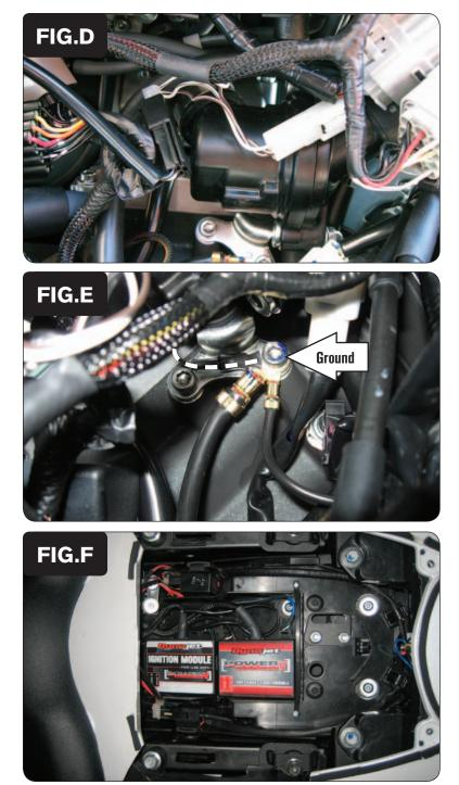
8 Plug the Ignition Module wiring harness in-line of the stock Crank Position Sensor connectors (Fig. D).
