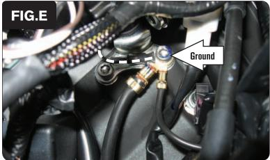
Attach the ground wire of the Ignition Module with the ring terminal to the stock common ground location on top of the engine case (Fig. E).
