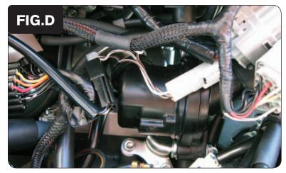
Plug the Ignition Module wiring harness in-line of the stock Crank Position Sensor connectors (Fig. D).
