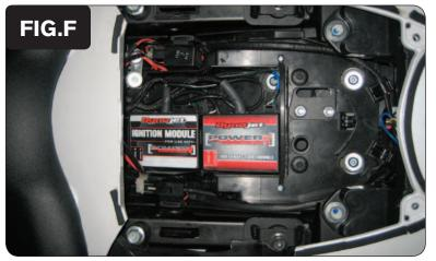
Plug the CAN link cable into one of the expansion ports on the Ignition Module and the other end into one of the expansion ports of the PCV module.
