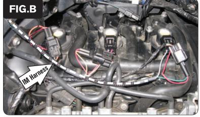
Plug the Ignition Module in-line of each coil stick and the stock wiring harness (Fig. B).
