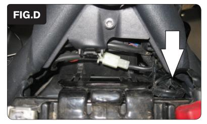
Move the fuse over to the right side of the battery compartment and tuck it out of the way (Fig. D).
