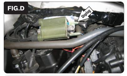
9 Unplug the BLUE/YELLOW wire from the ignition coil for cylinders 2 & 3 (Fig. D).
