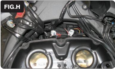
Plug the Ignition Module wiring harness in-line of the stock wiring harness and the front ignition coils (Fig. H).
