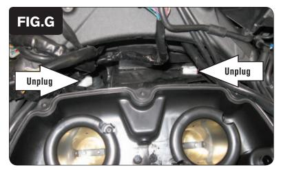
Locate and unplug the stock wiring harness from the front ignition coils (Fig. G).
