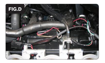
Plug the Ignition Module connectors in-line of the coil sticks and the stock wiring harness connectors (Fig. D).
