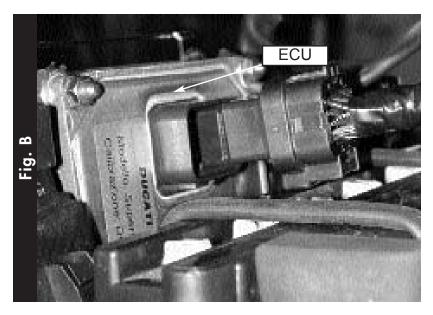
4 Plug male connector from PCIII into ECU (Fig. B).
