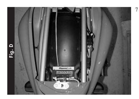
Mount PCIII unit to rear most area under seat using provided self adhesive velcro (Fig. D).
