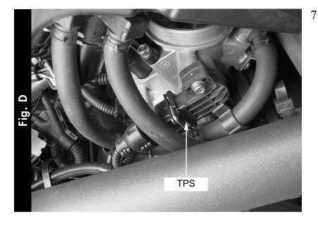
Locate the Throttle Position Sensor on the right hand side of the throttle bodies (Fig. D). Unplug the stock wiring harness from the TPS.
