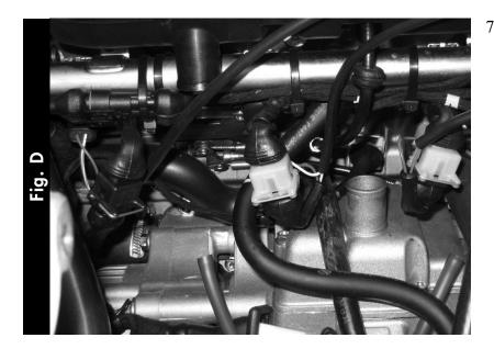
Plug the PCIII connectors in-line of the stock wiring harness and injectors (Fig. D).
