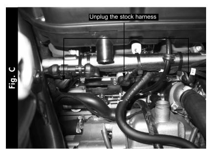
6 Unplug the stock wiring harness from each injector (Fig. C).
