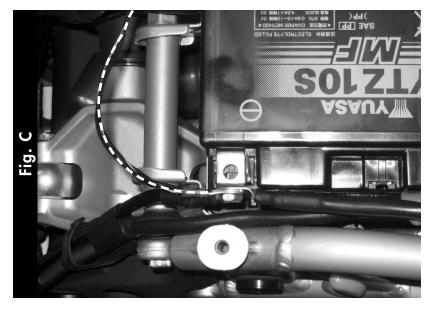
4. Connect the ground wire from the PCIII to the negative side of the battery (Fig. C).
