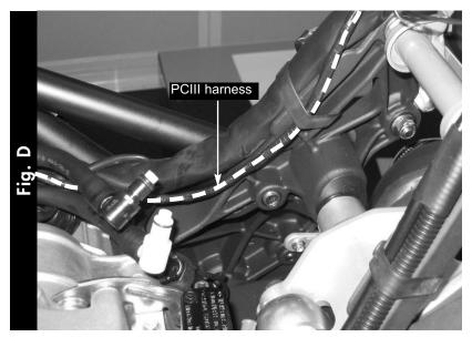
5. Continue routing the PCIII harness along the inside of the bike's harness towards the throttle bodies (Fig. D).
