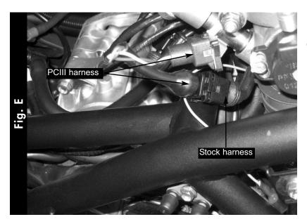
6. Plug the connectors from the PCIII inline of the stock injectors and wiring harness (Fig. E).
