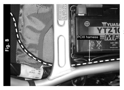
3. Route the Power Commander harness underneath the right side of the frame rail towards the front of the bike (Fig. B).
